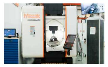
Mazak 5-axis machining centre VARIAXIS i-700. Its simultaneous 5-axis machining capabilities and our GARANT ZeroClamp system allow accurate processing of parts with complex profiled surfaces in a single setup.
