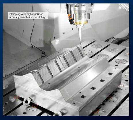
Using the GARANT ZeroClamp zero point clamping system will increase the productivity of your manufacturing. Long set-up times are a thing of the past. Reducing machine downtimes allows you to produce more components at a lower unit cost. If the measurement process shows the component needs further machining you can position the component on the machine quickly, precisely and with high repetition accuracy – be it for a small batch or a oneoff item.
