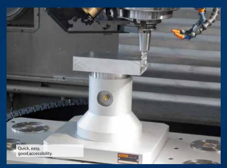
Quick and easy clamping using the GARANT ZeroClamp zero point clamping system: for instance NC vices secured to base plates by means of clamping studs, or (as illustrated) the workpiece is clamped directly to the clamping pot using an extension base.
