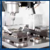
Clamping finished parts, e.g. using front pull-down jaws.
