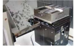
Blank parts are gripped directly and exchanged.
