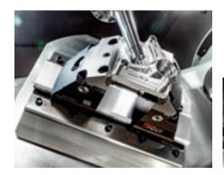
The **GARANT Xpent** offers flexible options for use on zero-point clamping systems. For the best possible stability, Hermle mount the vice on an adapter plate clamped to four clamping pots.
