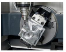
The **GARANT Xpent size 0** can be used on all Ø 320 mm turntables. The attachment is performed using stepless adjustable clamps or directly to the turntable using holes in the base rail.
