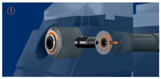
Disengage 2 locking pins per clamping module.
