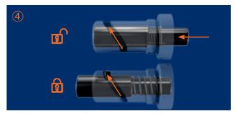
Push the pins in against the spring pressure until they engage.
