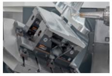
The 5-axis vice in conjunction with a 362 mm long base rail is very well designed for use on small turntables and pallet clamping systems.
