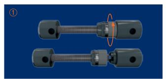
Release the union nut by hand. A spanner flat is provided in case a tool is needed to release the spindle.
